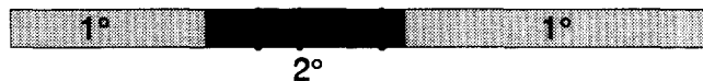
Fig. 1. Schematic representation of the procedure used to generate a pH gradient using a dynamic pulse: (A) Capillary rinsed with primary buffer ( 1^\circ ); (B) secondary buffer ( 2^\circ ) injected hydrodynamically; (C) analytes (black line) injected hydrodynamically and (D) electrophoretic separation assuming no broadening or inter-mixing of the buffer zones.
